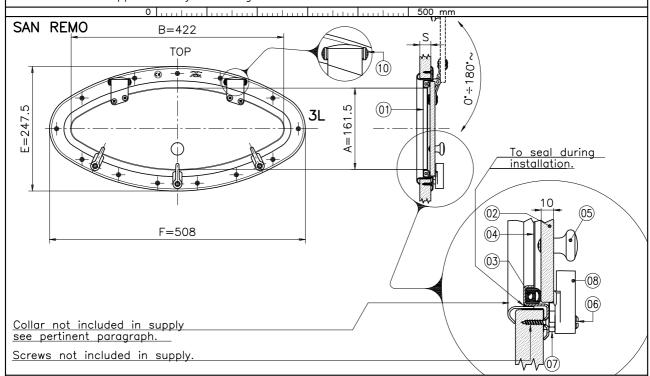
Portholes E.L. 160x 420: openable shutter, locking levers.
